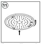
Align gear tray with screws and tighten
