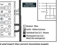
10) 5 Press the individual terminal and insert the correct incoming supply
