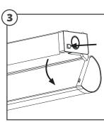
Push button on end-cap and pull open casing
