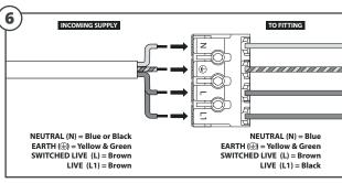
Push down the terminal, insert the correct supply (as above) into terminal block, for the emergency unit to work correctly please ensure that an uninterrupted permanent live feed is present and is connected directly to the (L1) "Permanent Live" terminal of the connector block. Release the push fit terminal to secure.
