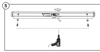
Drill screws into previously installed plugs
