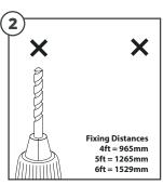
Drill holes to the required distance and install plugs
