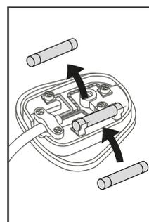
Remove 13-amp fuse and replace with an operational 13-amp fuse
